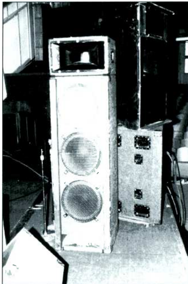
Figure 6. Side fill units have three-way driver systems and are five-feet tall.
